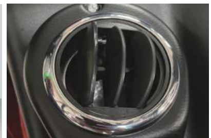
Dashboard with orientable heater outlet
